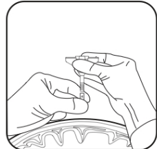
Figure 3: Select Bolt Stop size and slide onto bolt of the Bolt Assembly.
